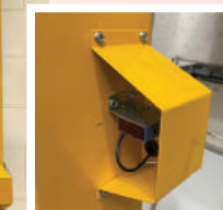
Photo-Electric Safety Beam Two 24v AC photo-electric safety beams fitted providing closing safety device, activated by breaking the beam IP65 Protection
